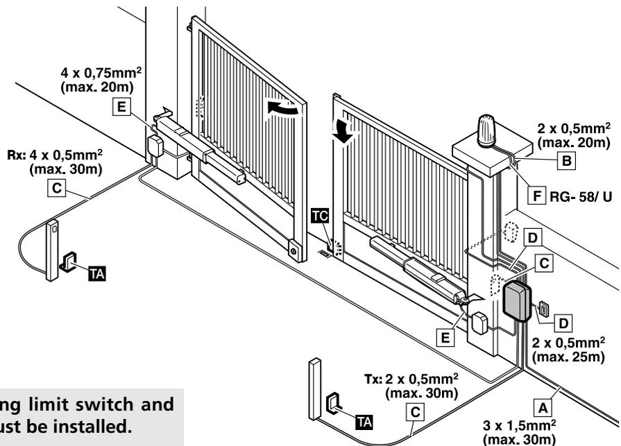
**VERY IMPORTANT:** The **TC** closing limit switch and the **TA** opening limit switches must be installed.
